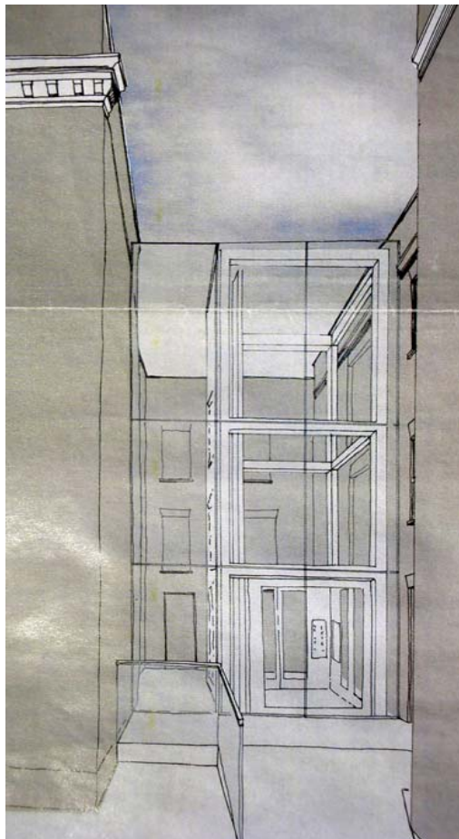
Glass lift in the yard by back door
